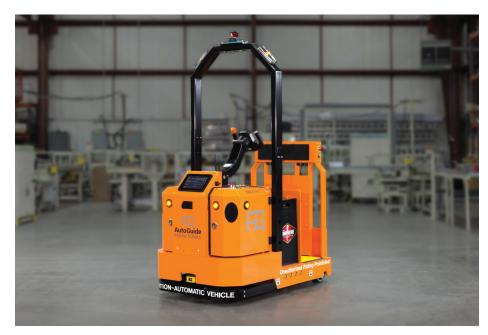
The Max-N15 Tugger is an automated tow vehicle that transports a train of trailers from point to point within industrial facilities. Standard towing capacity is up to 15,000 lbs. (6,804 kg).
